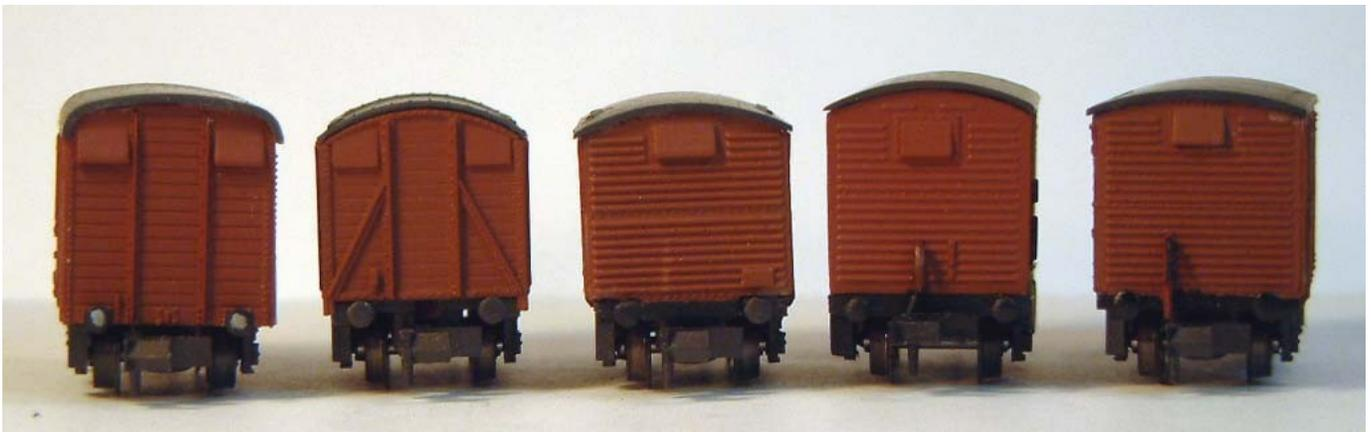
The SR design of van can nearly always be identified by the elliptical roof shape. The planked versions are the only vans that have diagonal braces on the sides that slope inwards from the bottom, all other vans with diagonal braces have them sloping the other way. SR vans were all
