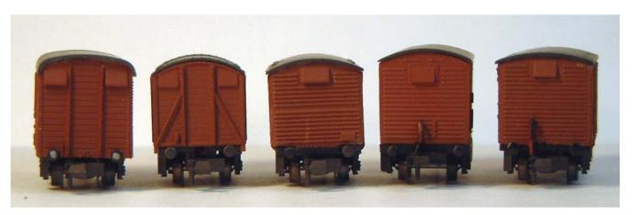
The SR design of van can nearly always be identified by the elliptical roof shape. The planked versions are the only vans that have diagonal braces on the sides that slope inwards from the bottom, all other vans with diagonal braces have them sloping the other way. SR vans were all
