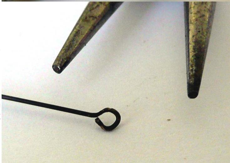
Make the hook part of the coupling by bending about 3mm at the end of the wire to rather more than 90 degrees, and then another slight bend about 4mm further down so the wire is at right angles to the end of the wire, as shown in the picture. After a few this is very easy to do by eye.
