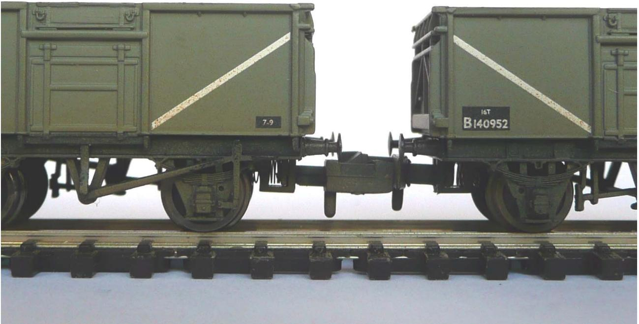
On many layouts rakes of mineral (and other) wagons will always run together, so automatic couplings are not needed and we can substitute a much smaller permanent coupling. This article shows how easy and cheap it is to make these couplings out of a couple of inches of wire, and have wagons that look like this:
