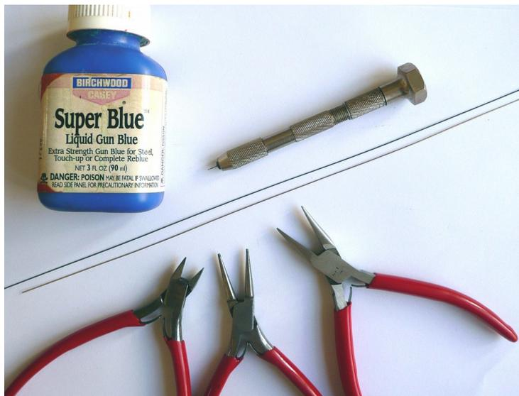
To blacken the wire first clean it by rubbing with a Garryflex block, or steel wool, or very fine wet and dry paper. Then coat with the blackening using a cotton bud, until suitably darkened. Wash excess off and let dry. Wipe with a bit of tissue moistened with ordinary mineral oil like 3 in 1 – this helps the coating harden. Leave overnight to harden.
