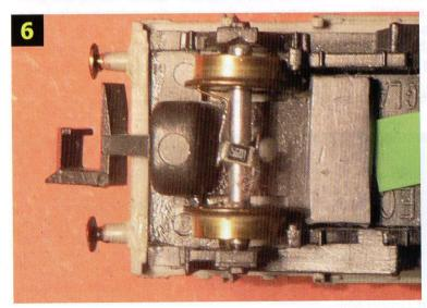
provided you add extra weight directly over the resistive axle so if the vehicle is only touching the rail at three points, as a 4-wheel wagon usually is, then both wheels of the resistive axle will be in contact.
