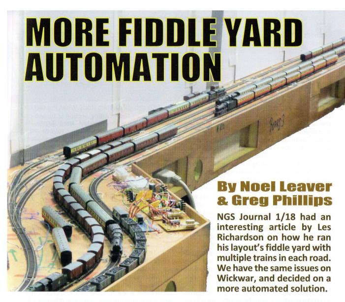
e wanted to minimise the space taken by the fiddle yard while still being able to store lots of trains. The best use of space is to have long roads with an automated 'shuffle' to move trains up. That is, a fiddle yard road with several trains in it and when the first is sent out the second moves to where the first was, the third to second, on so on. To allow a mix of long and short trains we wanted a train to be able to occupy more than one fiddle yard section.
