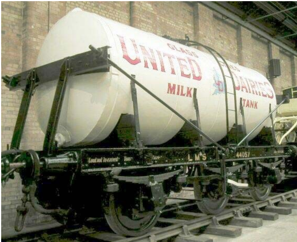
Milk Tank at NRM York. An LMS tank, note the 4 saddles supporting the tank and large coach wheels. The straps go under the outer insulation to the metal tank.
