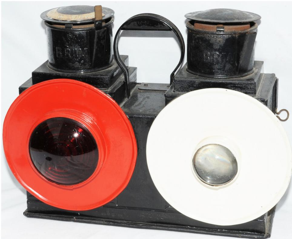
*A double lamp for the rear of the slip portion of the train, this arrangement of lamps was for the portion nearest the main train. To make them more visible the lamps on slip coaches had to have coloured disks round them.*
