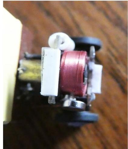
Photo 7 - 3mm magnet on top of original 1.5 mm magnet. It is pushed forwards, this adjusts the resting position of the arm which was over to one side and makes it straight. On the other side is a simple clip of a length of plastic tube with a slit to hold the actuator against the metal plate.
