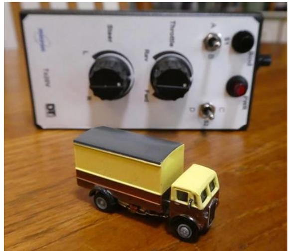
*Photo 1 - Lorry fitted with battery, receiver, motor, and steering. The transmitter I bought is behind.*
