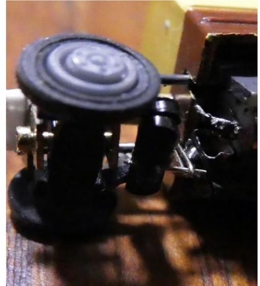
*Photo 5 (Left) - Brass sleeve over end of arm, with wire going down to steering and Photo 6 (Right) - 'Eye' in end of wire fits over a short wire inserted into the steering arm.*
