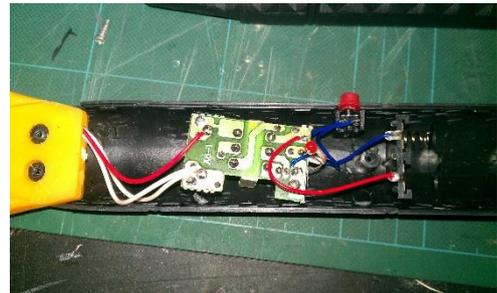
Bare the red wire to so that it's long enough to go around the tea strainer handle. If you can solder it to the tea strainer is better, but it's difficult to solder to stainless without a really good soldering iron. If you can't, then twist the bare wire around the handle and make sure the bare wire is touching the handle; solder it to itself and wrap some insulation tape around the handle and wire to make sure it's got a good contact.
