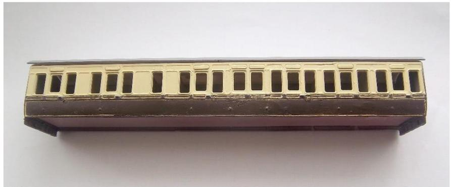
“The basis of the build is the Ratio U4 composite which has compartments of the correct length. 3 of these plus the luggage doors from a T47 brake van were cut and shut to form the body. The ratio ends are the right width and profile for the main roof, which itself is 2 lengths from the U4 cut and glued together and braced with plastikard.
