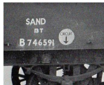
The yellow Circuit marking was to highlight that the wagons were allocated to and reserved for a particular traffic with details given below the arrow, such as 'To work between .... ' and 'Return empty to ...'. Later these details were moved to a yellow plate behind the label clip and the Circuit marking pointed to the label clip (on the lower left of the wagon).
