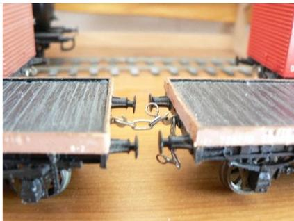
All the links are made from non-magnetic material such as half hard brass wire (24 swg) with the third link having a magnetic mild steel nail head soldered inside the loop. Extra solder has been added to the fixing of the nail head to the third link to increase the weight of the coupling and ensure that the coupling does not jump off its hook at speed !!!
