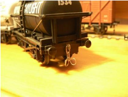
I tried several designs of having a loop of wire above the 3 links so they could be unhooked using an extended hook to lift the third link. This looks ok but the rolling stock could easily be lifted from the track and derailed.
