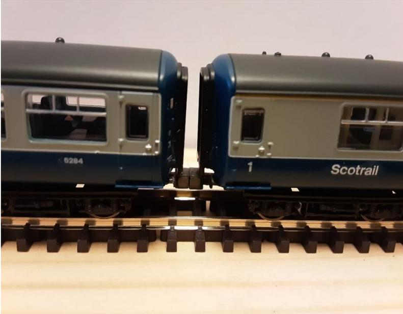
Recently, a new pack was introduced which claimed to be a replacement coupling for the Elsie coupling, as used by Peco. In fact these are a replacement for the early Graham Farish coupling which were held in their housing by a small spring. I have yet to try and fit one to a Peco wagon as it would appear that the 'T' end of the coupling will have to be reduced in width.
