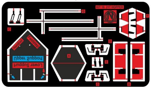
The black areas will not be etched, the white areas will be removed completely. The red areas will have the top half etched away, and the blue areas the underside half etched away. White in effect is red+blue, etch both sides away.
